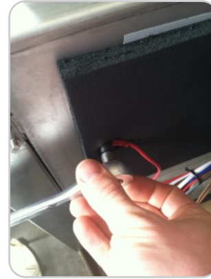
Step 3: Remove outer nut and wire Use the 7mm socket, to remove the outer nut and red wire.
