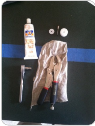
Step 1: Tools Needed Items: 7mm socket, vice grips, rag, silicone sealant, new sensor, emory cloth
