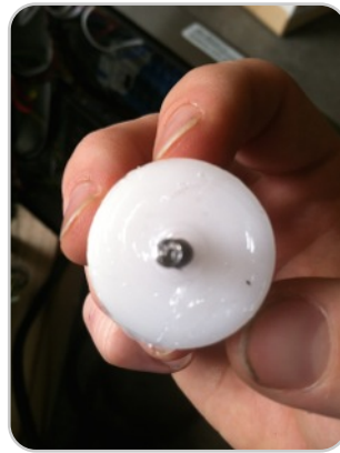
Step 7: Apply Silicone to new temp sensor Apply new silicone to the side of the white plastic where the threaded end of the sensor sticks out
