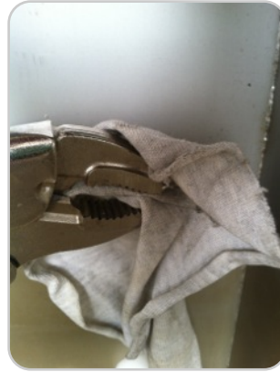
Step 3: Holding the sensor Use a rag to protect the end of the sensor and firmly lock onto it with a pair of vice grips
