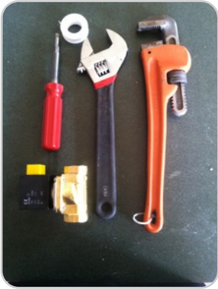
Step 1: Tools and supplies Items: crescent/pipe wrench, screw driver, Allen wrench, new valve, plumbers tape
