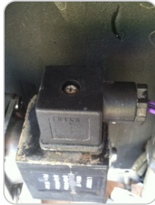
Step 3: Unplug connector Remove the screw in the top of the connector and unplug it.
