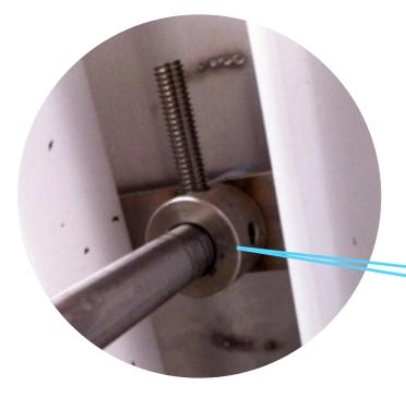
Collar location on each end of shaft inside the tank/bath
